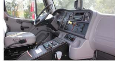
Custom communications console
