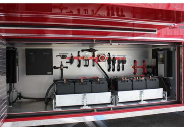
Batteries housed in slide-out locking trays
